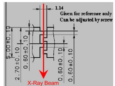
*Fig.2: Dimensional view of aperture*
