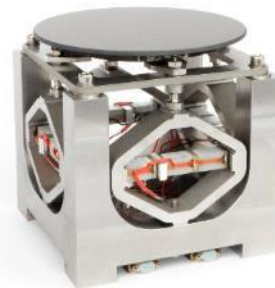
Figure 6: Piezo tip-tilt platform with 130 mm diameter light weighted rib structured HR-coated mirror
