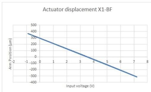
Figure 9: Mechanism displacement in closed loop.
