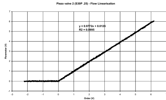
Figure.9 : Relationship between the order and the resulting flow (results monitored with a 8 byte numerical oscilloscope).
