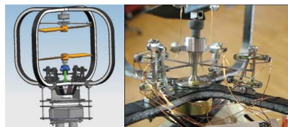
Fig. 14: CAD view of Mufly & zoom on actuators
