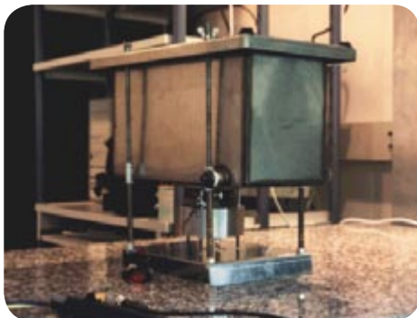
High power (3kW) magnetostrictive sonar transducer TRIPODE.
