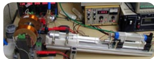
CEDRAT TECHNOLOGIES test bench of MRF in a flow mode (active valve mode).
