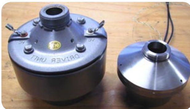
High power loud-speaker based on MICA concept (right) compared to the initial moving-coil loud-speaker (left). In this application, MICA offer 3 times more forces, twice more displacement, while requesting twice less power and being much smaller Courtesy of MADE.
