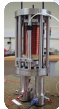
Magnetostrictive actuator for making an aircraft hydraulic pump in an Electro Hydraulic Actuator (EHA).
