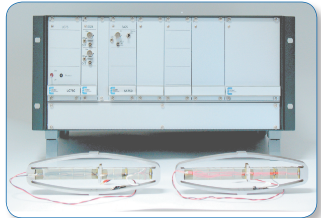
Fig: SA75D in Rack with sensor conditioner
