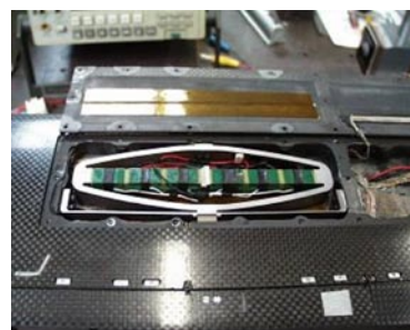
Helicopter Scale-1 blade with active flap including APA1000XL from CEDRAT TECHNOLOGIES.
