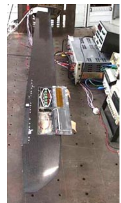
Helicopter Scale-1 blade with active flap including APA1000XL from CEDRAT TECHNOLOGIES.
