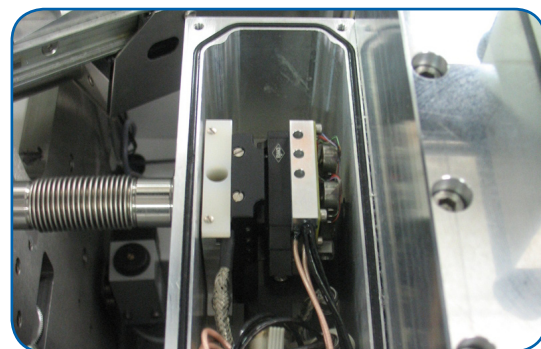
Figure 5: FPS 200M on a XY stage on a MX Beamline (Courtesy ESRF)
