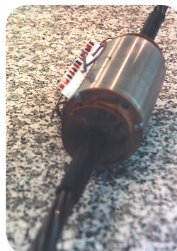
Figure 3: Design and assembly of the sensor around of the cable.
