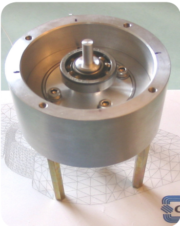
Figure 2: Frame with rotor and stator
