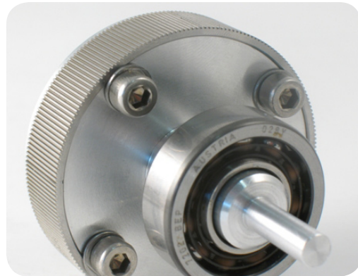
Figure 4: Shaft with rotor and bearing
