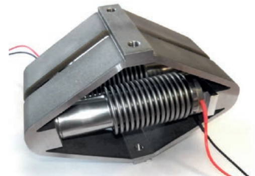
Fig. 5: Example of piezo ceramic encapsulated with bellows assembly
