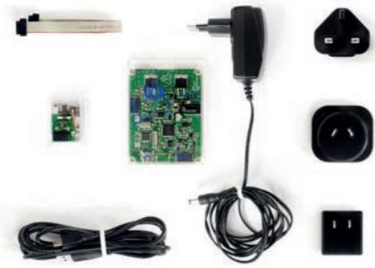
Fig. 5 : Components of the LSPA30uXS developer kit
