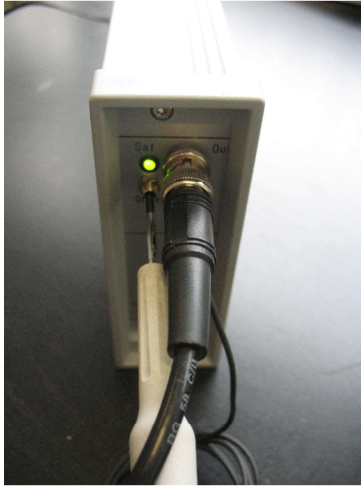
Figure 3-8: Setting the offset of the BNC output.
