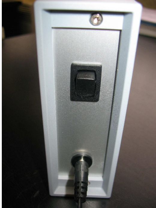
Figure 3-2: AC/DC adapter connection on the rear panel.
