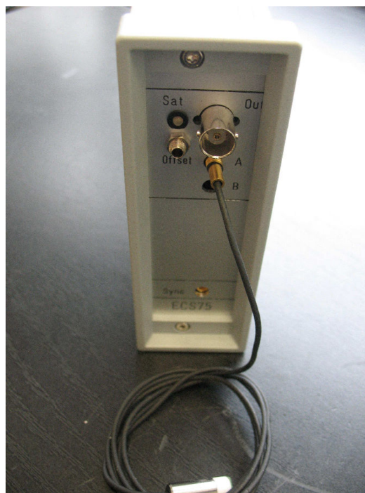
Figure 3-1: Probe connection on the front panel.
