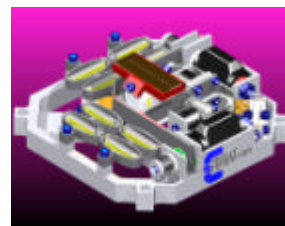
Figure 10. IDEAS CAD view of a piezoelectric XYZ stage qualified for the Rosetta/Midas instrument
