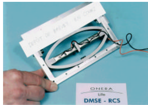
Figure 16. Helicoptere flap segment based on the APA230L, as designed by Onera
