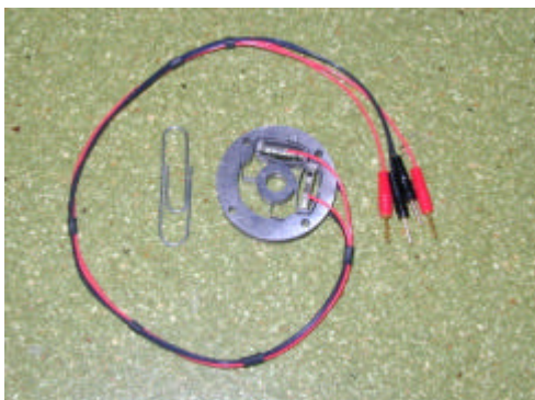
Figure 13. XY mechanism based on 2 APA25XS
