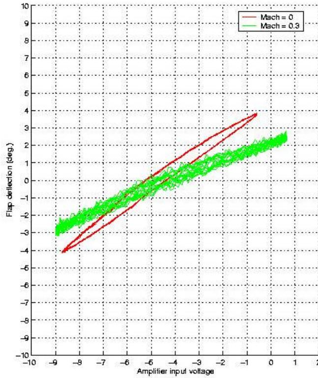
Figure 3 – Influence of aerodynamic loads on flap deflection
