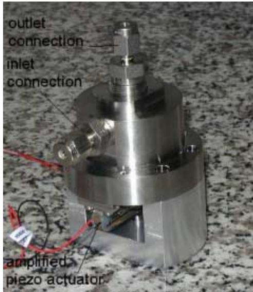
Figure 2 : Photograph a second piezo actuated valve.
