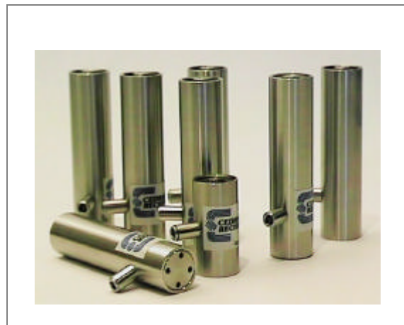
Figure 2 – Direct piezoelectric actuators DPA90 (longest one) based on a 1cmx1cm section 9cm long MLA, offering more than 100µm stroke (Cedrat Technologies products [21])
