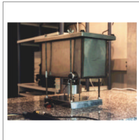
Figure 4 – High Frequency Magnetostrictive Transducer for Ultrasonic Cleaning Source - R&D project Cedrat-Feredyn (ECAMMA coord. by Syncom)
