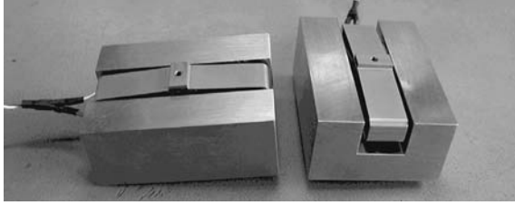
Fig. 1: Electromechanical device built around APA400M-MD
