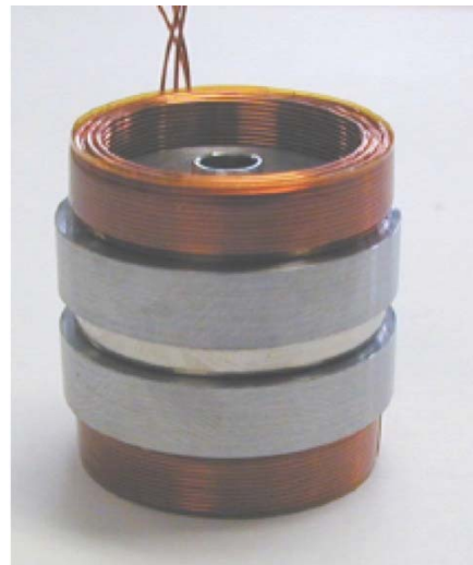
Figure 2 : View of the magnetic head for the MRF based shock absorber.
