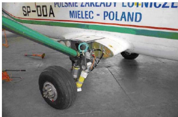
Figure 8 : View of the PZL aircraft equipped with the adaptive landing gear.
