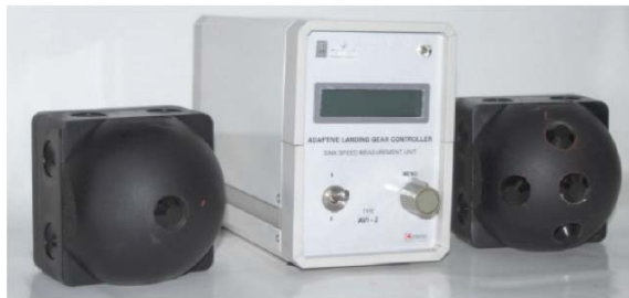
Figure 4 : View of the ultrasonic speed sensor.
