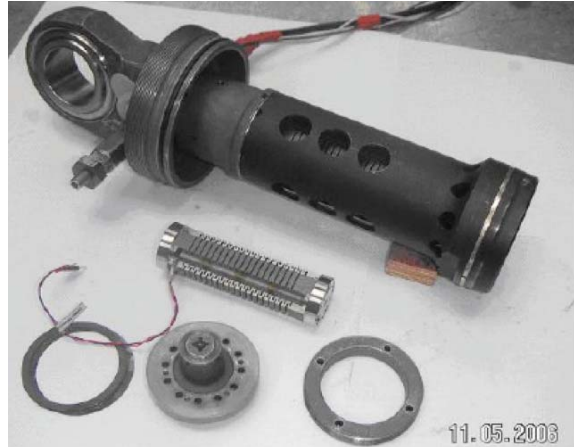
Figure 1 : View of the shock absorber including the piezoelectric valve.
