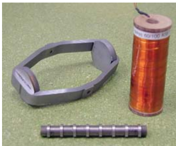
Fig.3: Dismounted PM biased AMA400L
