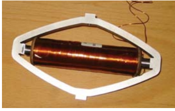
Fig.5: AMA230L preloading actuator for TPMA
