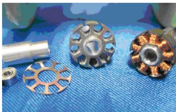
Figure 1: View of the BLDC parts
