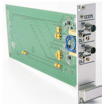
Figure 10 Electronic conditioner card for eddy current sensors
