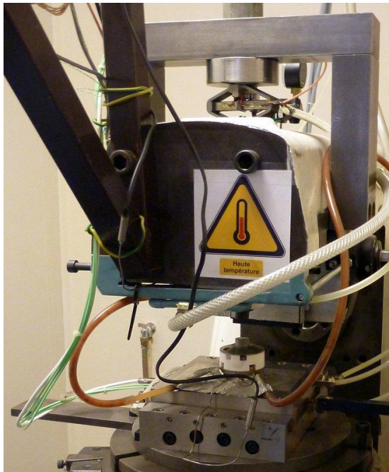
Fig. 8 IMPACT II: APA120ML actuator for impact or normal force control (Courtesy of LAMCOS)
