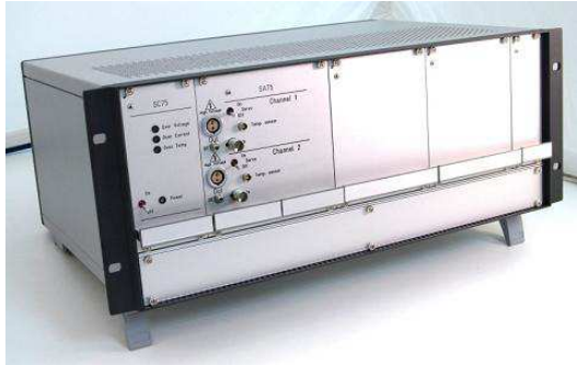
Figure 4: SA75D assembled in standard 19 inches rack.
