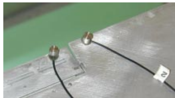
Figure 12 – Accelerometers on airfoil and flap (at rest)
