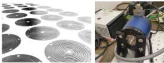
Figure 5 Flexure bearings fatigue test running since 2017
