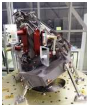
Figure 5. IASI NG Interferometer Mechanism (Courtesy of Airbus DS)
