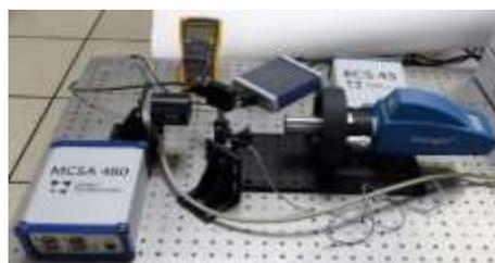
Figure 5 Optical test bench with ECS45 and MCSA480
