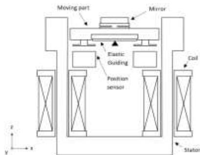
Figure 3 M-FSM structure (ZX cross section)
