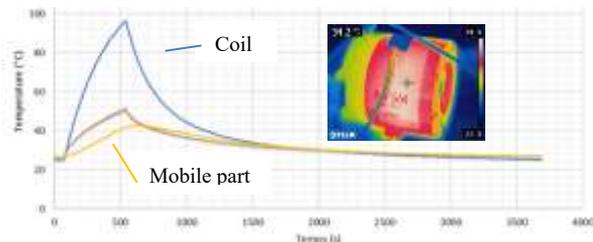
**Figure 7** Heating at 10Apk 200Hz drive
