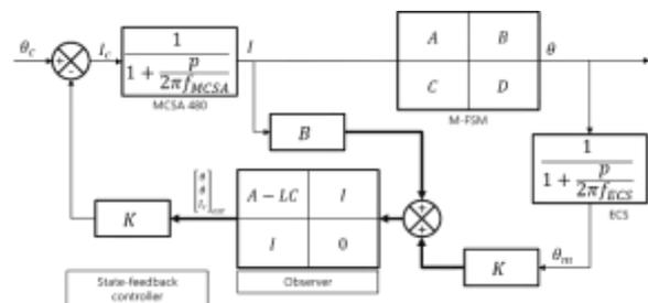
**Figure 10** Controller architecture
