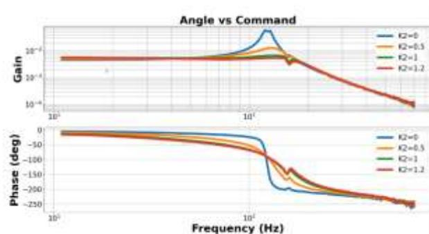
**Figure 12** Experimental results of the controller (achieved damping)
