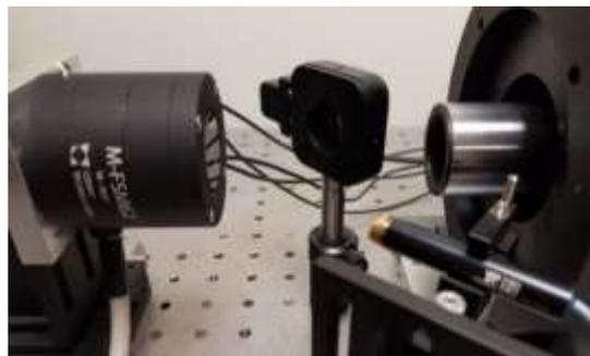
**Figure 2** M-FSM62 EM on optical test bench
