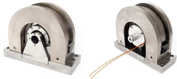
Figure 9 : The test bench of the RCVM-180 motor
