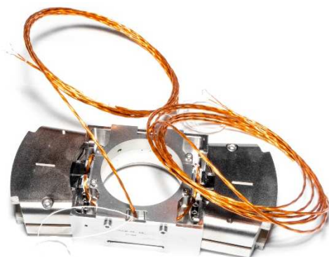
Figure 2 : The RVCM – MTG scan mechanism
