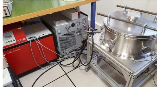
Figure 13 : Cryogenic vacuum test bench
