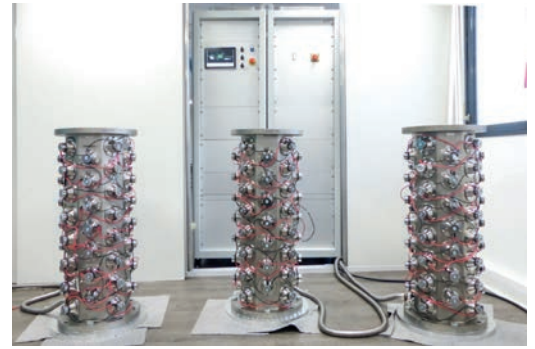
Fig. 3: Command/control electronics, drivers and three US vessels each fitted with 60 transducers.
