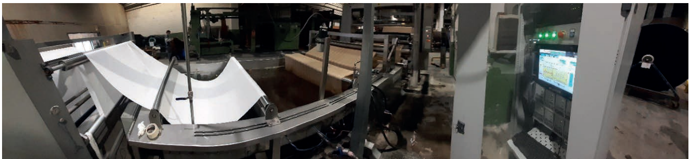
Fig. 1: R2R machine with 1.5 m width ultrasonic Tank for cotton Fabrics. The brown color is the coating results.
