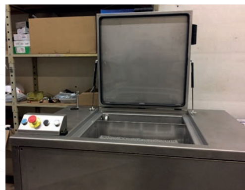
Fig. 3: Batch Tank for Catheters Sonication
