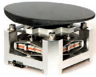
Fig. 17 : FSM with non-coated SiC mirror
