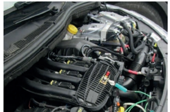
Fig. 2: e-Lift3 ElectroMagnetic Actuators integrated in a 3-cylinder thermal engine
