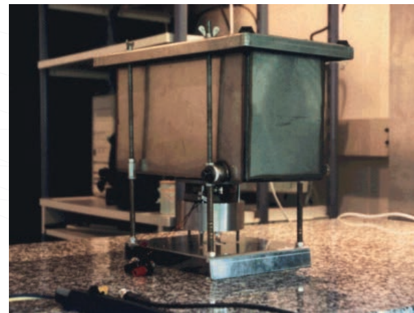
Fig. 3: High power (3kW) magnetostrictive sonar transducer TRIPODE.
