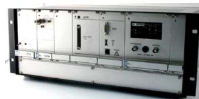
Human Machine Interface with LabView® software and rack84F including a Unit Control UC75 based on Compact-RIO product.
