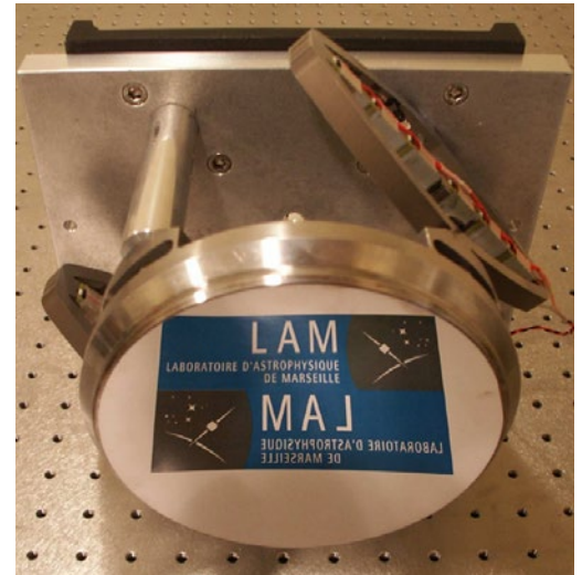
Fig. 4: The Beam Steering Mirror with APA230L
