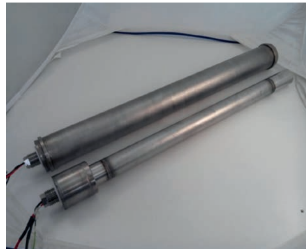
Fig. 2: Photo of both modular (MUST) [top] and conventional UST [bottom]
