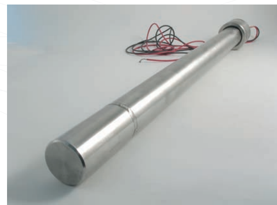
Fig. 2: Prototype of classic tubular ultrasonic transducer
