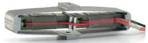
Fig. 2: APA 400M Displacement=400µm Blocked Force=38N Stiffness=0.1 N/ µm Blocked-Free resonance frequency=495 Hz.
