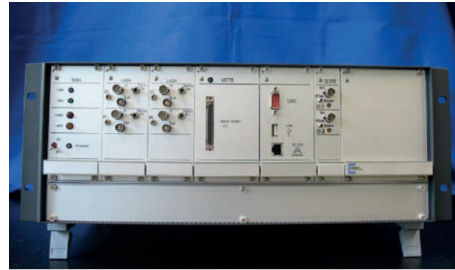
Fig. 1: View of rack including a Switching converter SC24, a Linear Amplifier LA24-2, a UC75 real time controller and a Eddy Current Sensor ECS75-2
