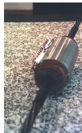
Fig. 3: Design and assembly of the sensor around of the cable.
